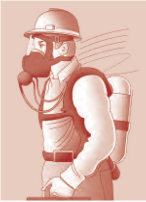
Full Facepiece SCBA Pressure demand mode is APF=10,000 Needs to be fit tested
