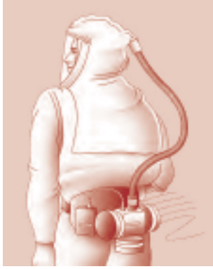
Hood Powered Air-Purifying Respirator (PAPR), APF= 25
